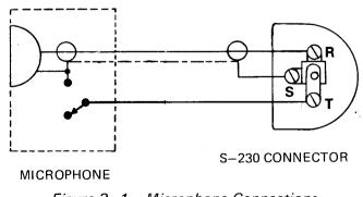
Figure 2–1. Microphone Connections
