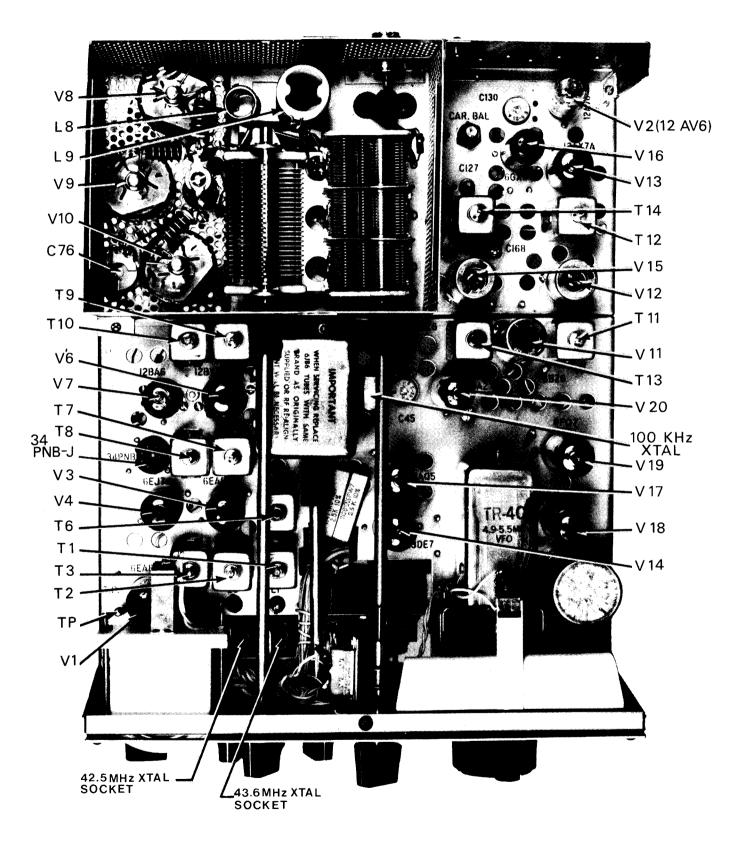
Figure 5-1. Alignment Locations, Top View
