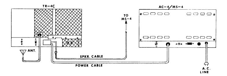
Figure 2–6. Connecting the AC–4 Power Supply and MS–4 Speaker
