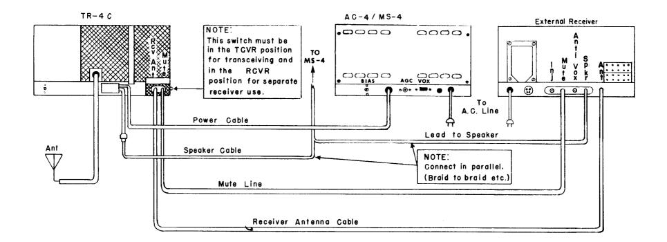
Figure 2–9. Connecting an External Receiver
