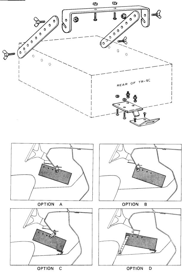
Figure 2–4. Mobile Installation Mounting Options
