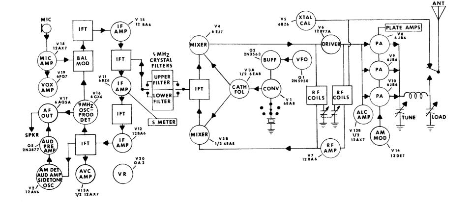
Figure 4–1. Block Diagram
