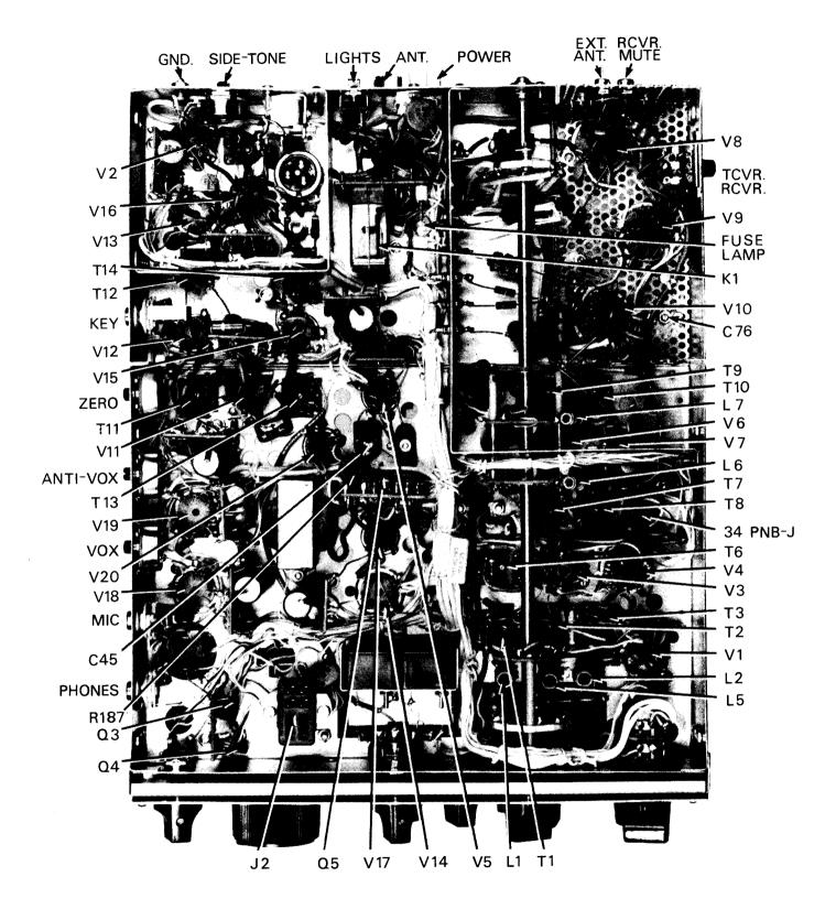
Figure 5–2. Alignment Locations, Bottom View
