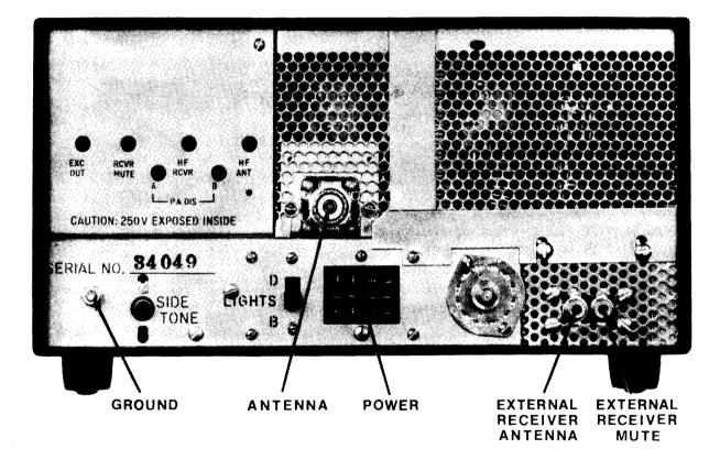
Figure 2–2. Rear Chassis Connectors
