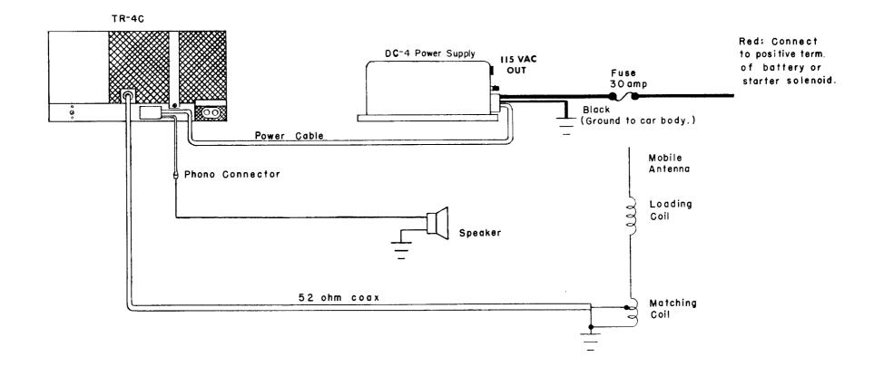
Figure 2–3. Electrical Connections Required for Mobile Installation
